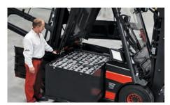
**Battery change with hydraulic battery replacement system** The battery lifts out of the truck hydraulically by up to 60 percent at the touch of a button. The battery can then be removed using an overhead crane.
