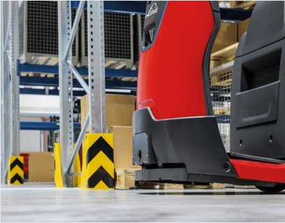
Linde BlueSpot™ and bumper including safety scanner
